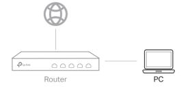
Connect a computer to a LAN port of the router with an RJ45 cable properly. If your computer is configured with a fixed IP, change it to Obtain an IP address automatically.
