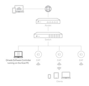
1. On the PC with Windows OS or Linux OS, download the Omada Software Controller installation file from
